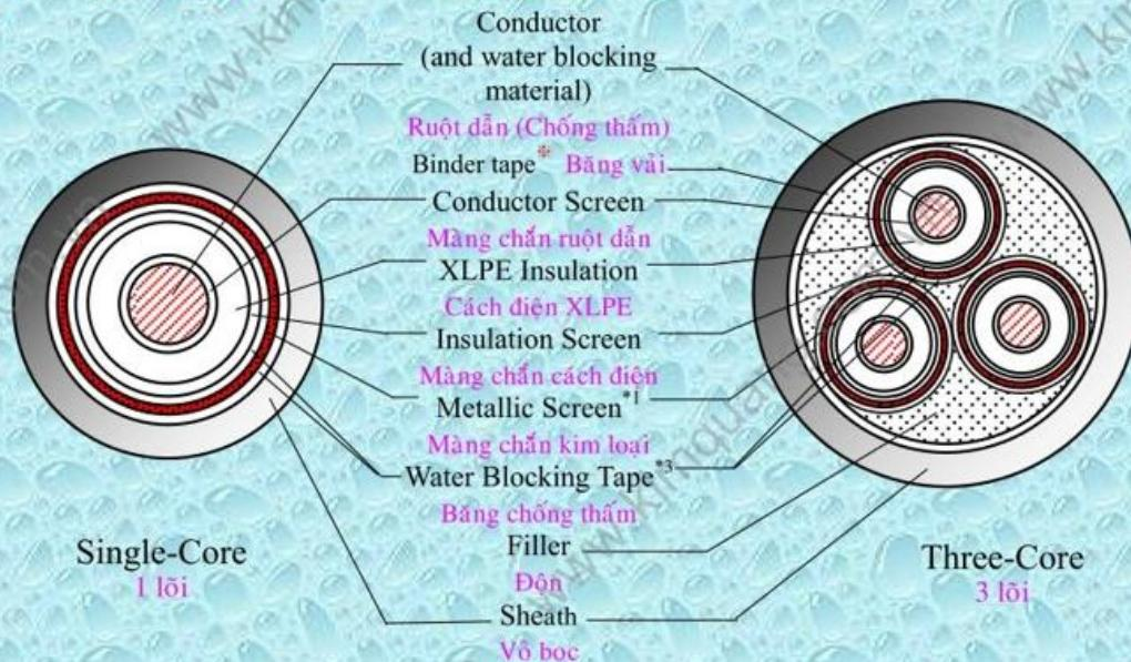
➤ **Armoured Cables With Water Blocking Function:**
